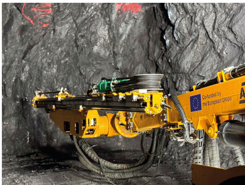
The boom of the DINAMINE jumbo during test drilling at the Skaland Graphite mine.
