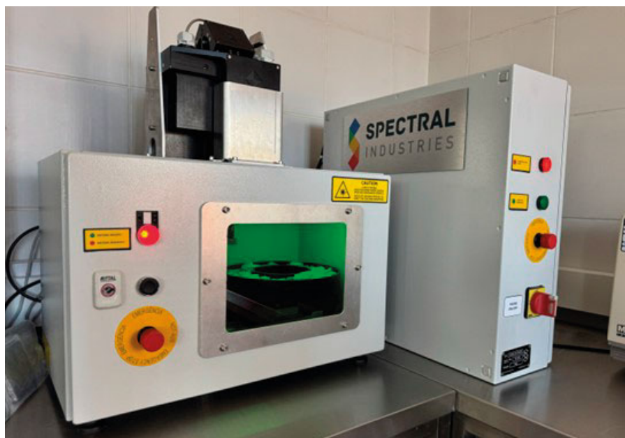
LIBS Lab analyzer installed at the lab of Felmica processing plant for the monitoring of elemental concentration in the primary product.
