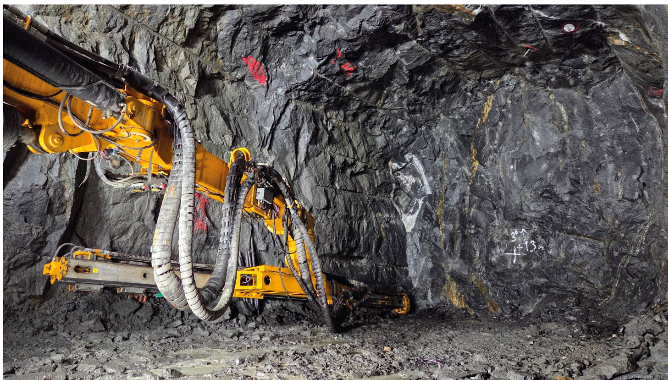
The boom of the DINAMINE jumbo during test drilling at the Skaland Graphite mine.
