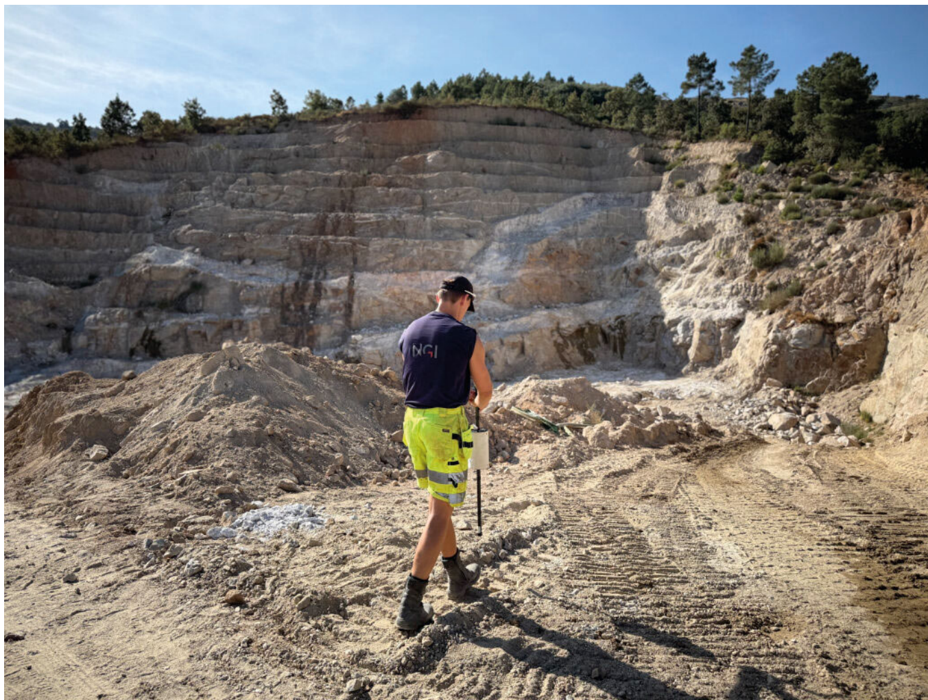
The final DINAMINE exploration campaign used GPR and ground magnetic geophysics for near-mine mapping of pegmatite deposits
