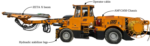
Fig. 1. AMV drill jumbo with one articulated arm.
