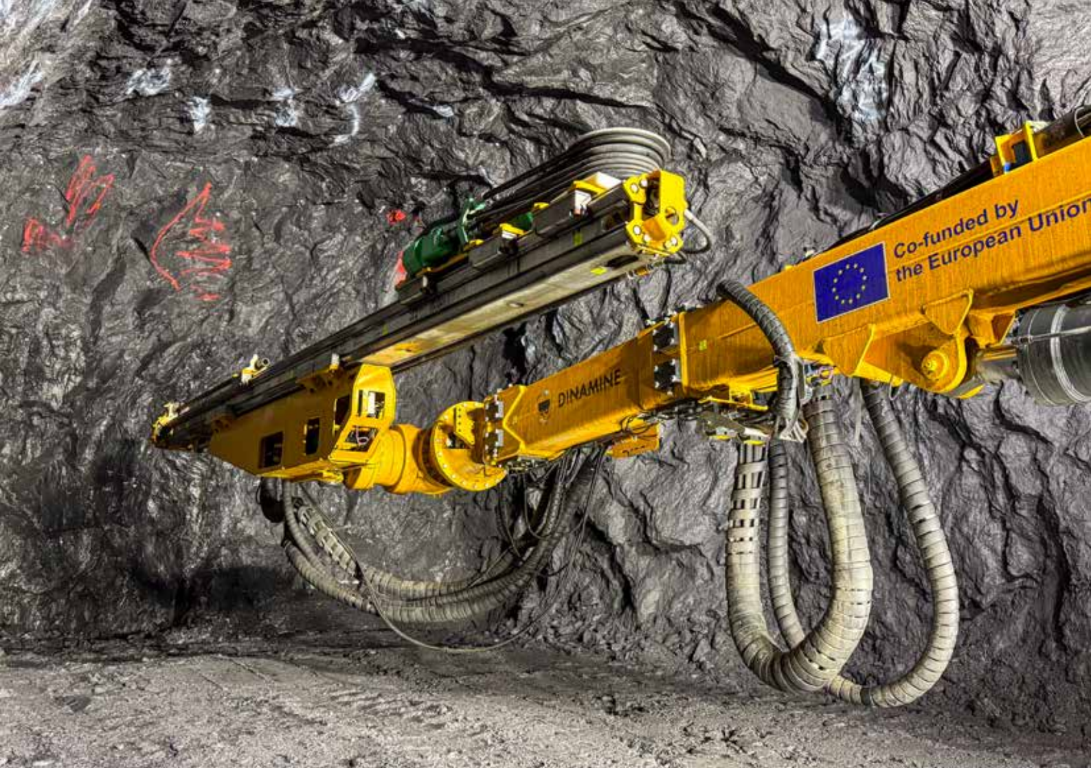
Figure 2 - The boom of the DINAMINE semi-automated drilling jumbo operating underground at the Skaland Graphite mine in Norway.
